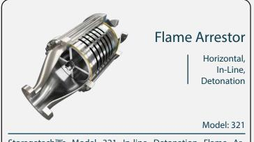
Storagetech<sup>™</sup>'s Model 321 In-line Detonation Flame Arrestor (also called flame arrestor or fire arrestor) is designed for installation in gas pipelines. Detonation occurs when a flame travelling through the pipeline reaches supersonic velocities, usually as a result of the pipeline configuration or pipeline surface roughness. Changes in gas density and pressure causes the flame velocity to metamorphose from subsonic to supersonic.
