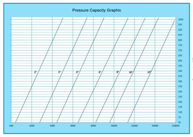
Maximum Flow Capacity (m³/h)
