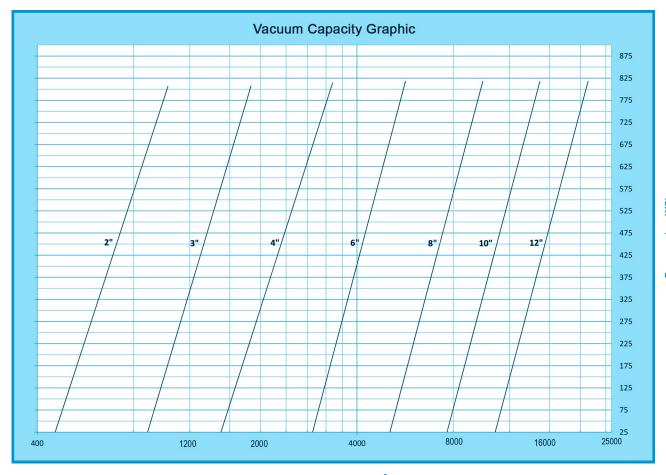
Maximum Flow Capacity (m³/h)
